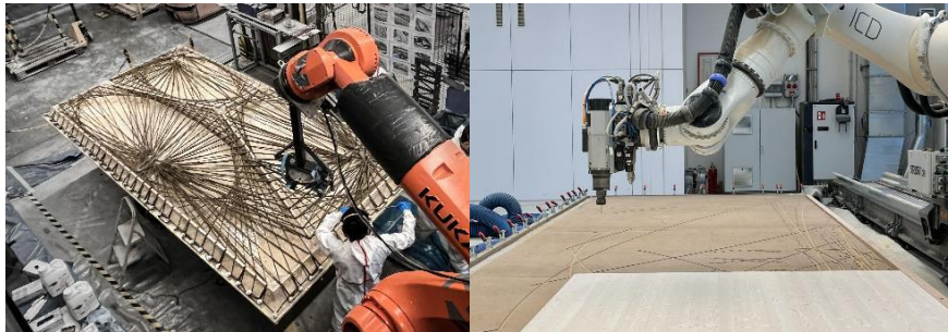
Figure 10. Winding process (left), and timber milling process (right) ©ITKE University of Stuttgart © ICD/ITKE University of Stuttgart
