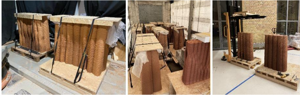
Figure 7. Pieces drying during shipping (left). Transport of 3.2Tn (center). Stacking of pieces (right) © IAAC 3DPA 2022-2023
