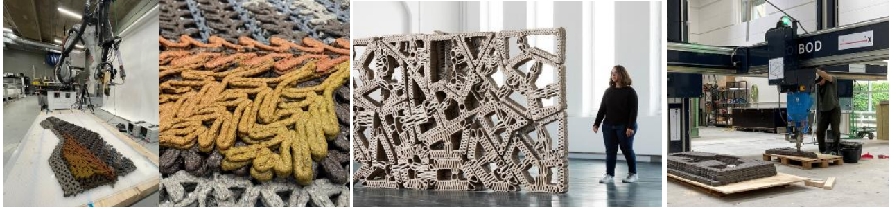
Figure 3. The grading of the cellulose source (e.g. recycled paper, bark, linen, cotton) as well as to the binder (Xanthan or bone glue) can create a variety of material expressions and behaviours. International Academic Workshop of CITA at 2022 ACADIA conference - Penn University (left). Cellulose Wall demonstrator exhibited in Copenhagen (2021) @Anders Ingvarstsen, Printing of Cellulose Screens on the COBOD BOD2 542 gantry 3D-printing system - June 2022 @CITA (right)
